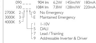
Please note, different colour appearances (K) of LEDs have slightly different lumens outputs, so, using various manufacturers figures DAL quotes mean average lumens for L and C products.
